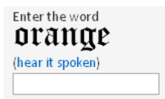
An early day example of CAPTCHAs before people started distorting the text (Atwood 2007). What makes this good is that it is easy to read whilst serving its purpose. The unfortunate thing is that it can be broken by a programmer in a short period of time.
